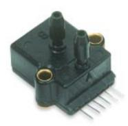
The SCX series sensors provides a very cost effective solution for pressure applications that require high accuracy over a wide temperature range. These internally calibrated and temperature compensated sensors were specifically designed to provide an accurate and stable output over a 0°C to 70°C temperature range. This series is intended for use with non-corrosive, non-ionic working fluids such as air, dry gases and the like.
