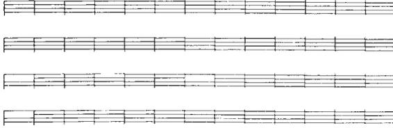
In this example, some of the nozzles are clogged, resulting in a void in the print. You would run the head clean procedure, then run the print sample again.
