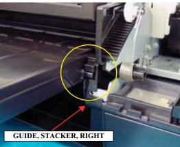
Figure 4-58. Removing the STACKER, ASSY.
