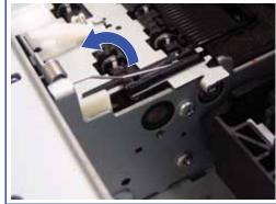
Figure 4-71. Tilting the FRAME, PAPER, EJECT, ASSY
