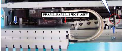
Figure 4-74. Tilting the FRAME, PAPER, EJECT, ASSY
