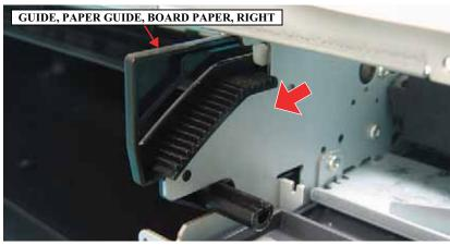
Figure 4-70. Pulling out the GUIDE, PAPER GUIDE, BOARD PAPER, RIGHT
