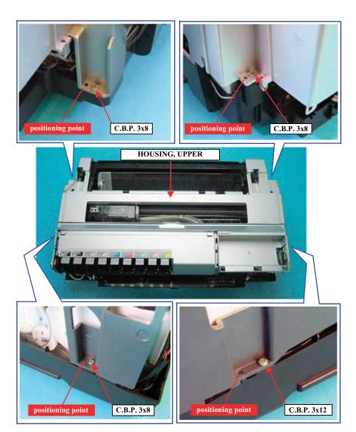
Figure 4-19. Removing the HOUSING, UPPER
