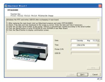
Figure 5-11. [RTC&USB ID] Screen (1)
