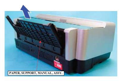
Figure 4-12. Removing the PAPER, SUPPORT, MANUAL, ASSY.
