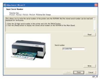
Figure 5-37. [Input Serial Number] Screen
