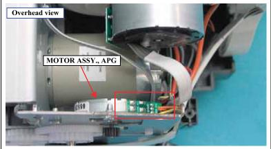
■ The screwing portions of the MOTOR ASSY., APG must come to the outside of the main frame.
