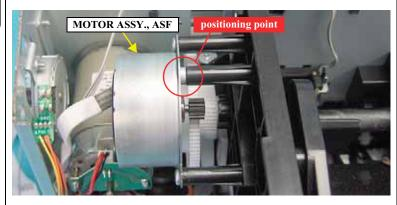
■ Secure the grounding terminal and the MOTOR ASSY., ASF together with the C.B.S. 3 x 8 screw at the rear as shown in *Figure 4-42*.
