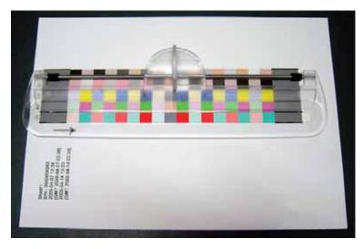
Figure 5-50. Setting the Chart and the Scanning Ruler
