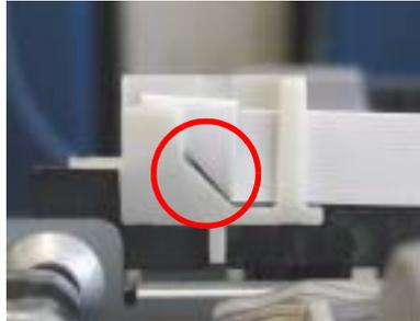
Figure 4-23. Installing the Head FFC
