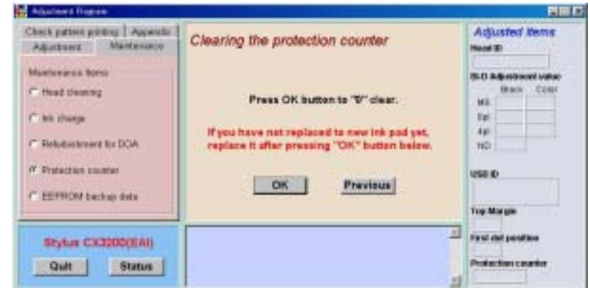
**Figure 5-15. Clearing the Protection Counter**
