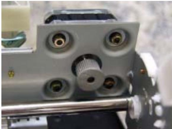
Figure 4-33. Removing the CR Motor
