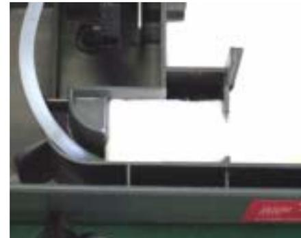
Figure 4-28. Removing the Tube Holder Waste Ink Pad
