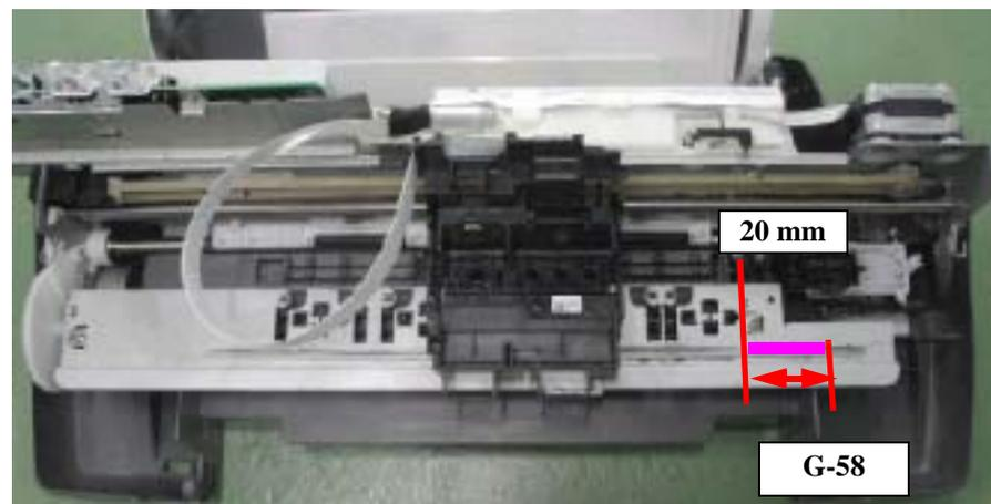
Figure 6-5. Lubrication Points of the Printer 4
