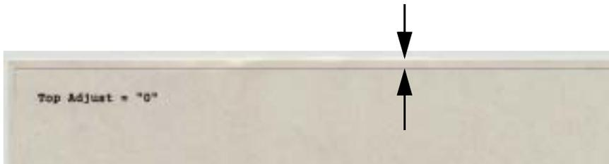
**Figure 5-10. Top Margin Adjustment Pattern**
