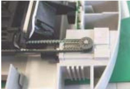
Figure 4-13. Driven Pulley for Timing Belt
