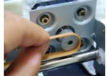
Figure 4-30. Removing the Timing Belt
