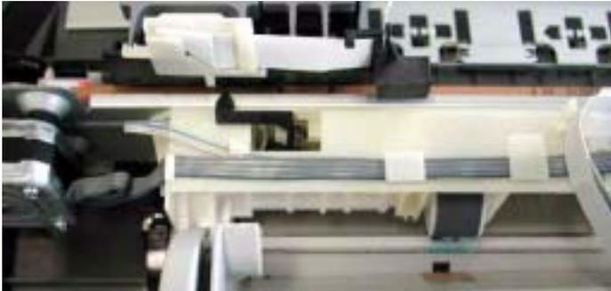
Figure 4-32. Releasing the Motor Lead Wires
