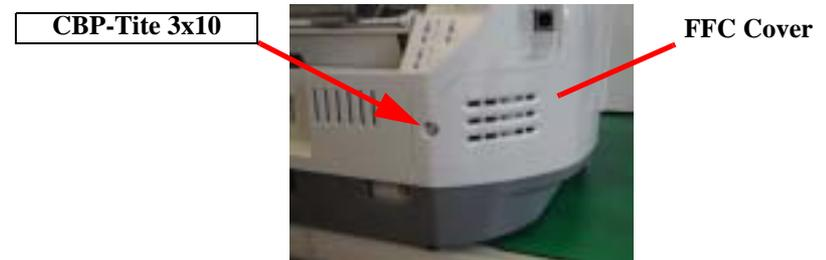
Figure 4-2. Screw securing the Connector Cover
