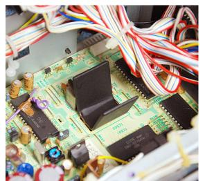
vious page (smaller arrow). At left is a closer view. It is formed from 0.0625" copper sheet metal. I obtained the material by splitting copper water pipe but that is the hard way. The heatsink should be painted flat black. Odd as it may seem to those not familiar, the paint improves emissivity. However, you should mask the surface which contacts the
