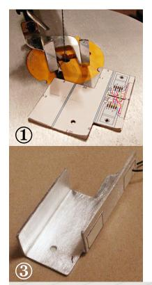
At left, the sheet metal is cut using a scroll saw with a metal-blade. I used a paper template, pasted to the metal. Not sure if that was really better than just scribing the piece. The example here is the DIY replacement amp version but the original amp version is similar. The main difference is in adding a slot.<sup>1</sup>
