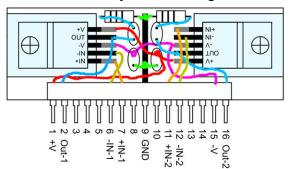
reversed relative to the view from the component side. Use the un-reversed diagram at left, the photo below and the schematic as wiring guides.
