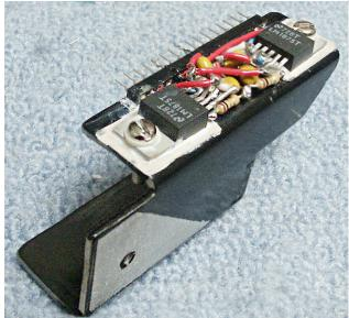
As shown <u>at left</u>, the servo amp is constructed on the aluminum heatsink. Of course, the circuitry is added after the heatsink has been cut, bent and painted.
