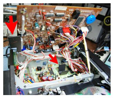
To improve heat dissipation, the left, upright panel of the heatsink is flush against the rear panel of the player chassis. Part of the horizontal area in the foreground overlays an existing horizontal bulkhead. It could be screwed to that for additional cooling. I did not find that necessary, though. With this heatsink in place, it and the amp module only get modestly warm to the touch, a big improvement.
