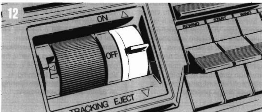
Set the ON/OFF/EJECT lever to the OFF position.
