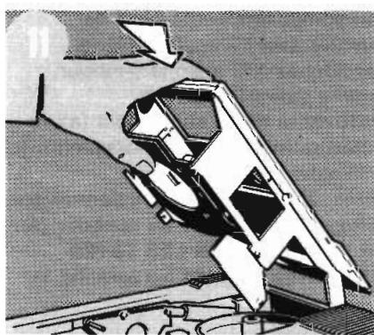
Replace the cassette holder (taking good care not to touch the head drum) and press the cassette holder back into the VCR.
