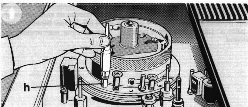
Using the hollow end of the cleaning gadget, clean the larger guide pin (h).
