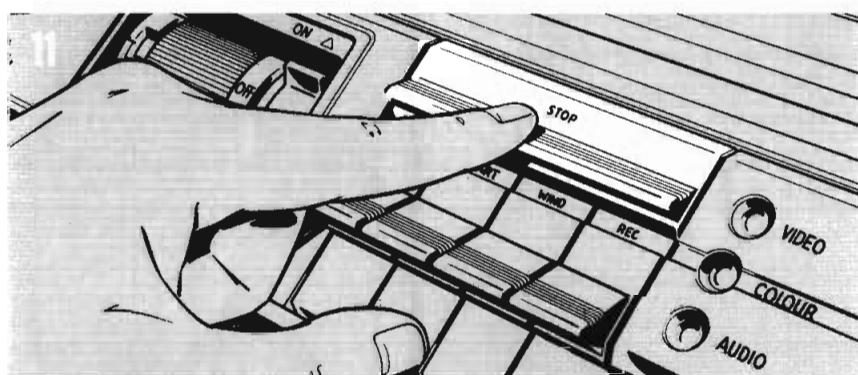
Press the STOP bar. You have now made a test recording that can be used to tune your television set by following the instructions given in Steps 11 to 24.
