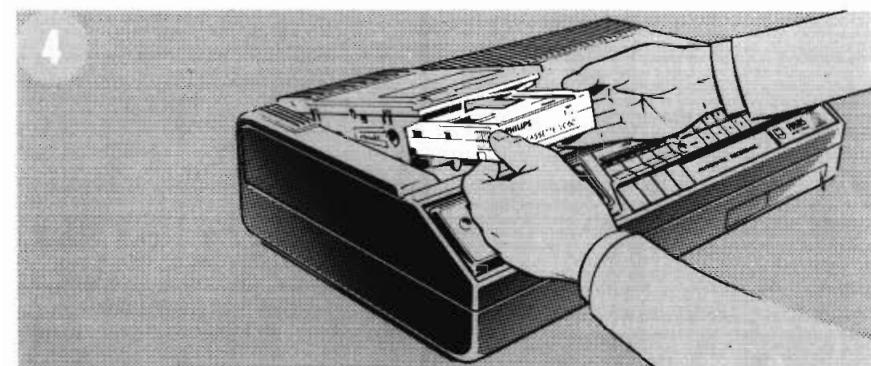
Press the ON/OFF/EJECT lever of the VCR downwards (▼) to release the cassette holder.
