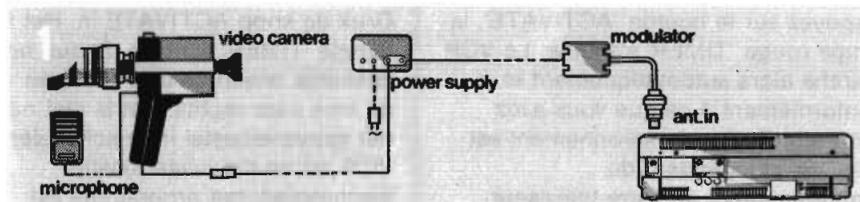
Connect the camera to the VCR using the interconnection cable(s) shown. Any video camera with an r.f. output may be connected in this way.
