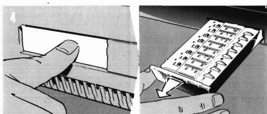
Push the left-hand drawer on the front of the VCR to release the catch, then pull out the drawer.
