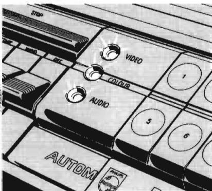
Turn Tuning Wheel 1 on the VCR until the VIDEO lamp lights. It indicates that a television channel is being received. The intensity of the AUDIO lamp varies with the rhythm of the audio signal of the programme. If the COLOUR lamp lights, the programme is in colour. Finely tune Tuning Wheel 1 to find the mid-position of the range over which the VIDEO lamp is lit. Push the drawer back to the closed position.
