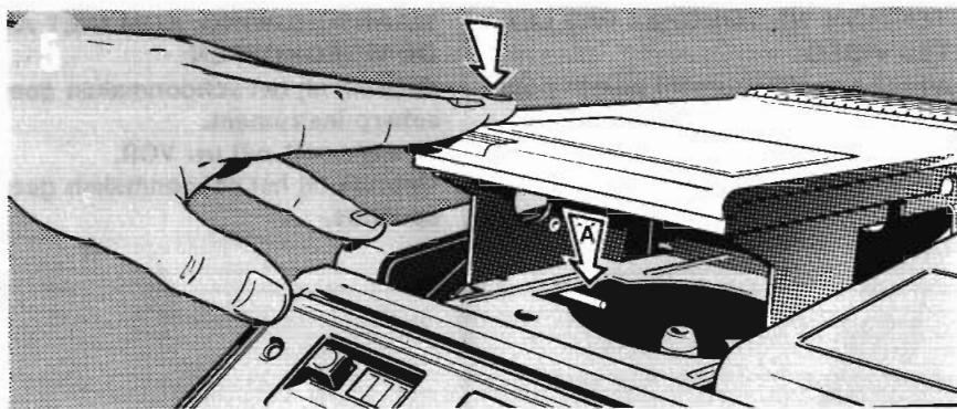
Press the cassette holder downwards halfway and with the other hand push pin 'A' down. Allow the cassette holder to rise again.
