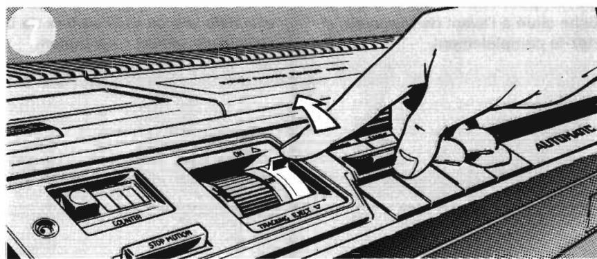
Set the ON/OFF/EJECT lever to the ON position (▲).
