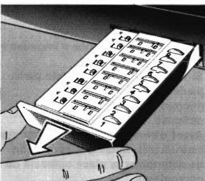
First push the left of the two drawers on the front of the VCR to release the catch, then fully pull out the drawer. Prepare both the camera and the sound source for use and switch on the TV set before continuing with Step 6. Press the last pre-selector which has been prepared for use with the VCR (see Page 52 Step 15).
