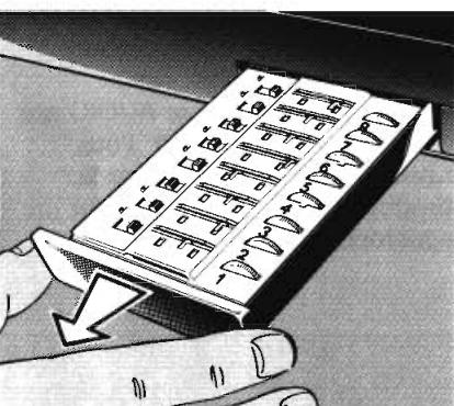
Push the left-hand drawer on the front of the VCR to release the catch, then pull out the drawer.
