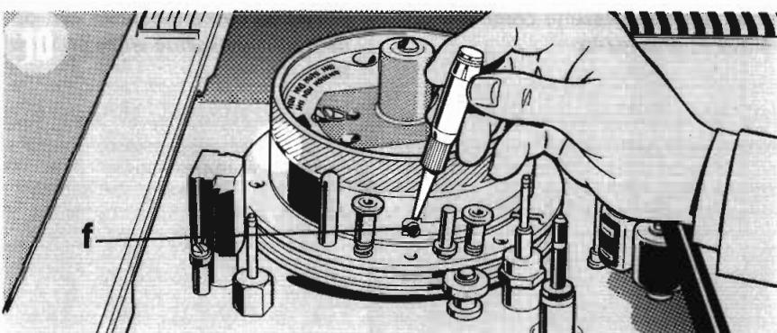
Using the thin end of the cleaning gadget, clean the top of the guide cam (f).
