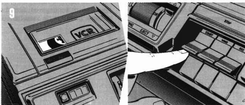
If the tape reel of the cassette (as seen through the cassette holder window) is empty, the tape has been completely rewound. If not, press the REWIND key to wind the tape to the beginning. Wait until the REWIND key automatically springs back.
