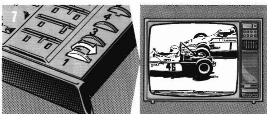
Adjust Tuning Wheel 1 on the VCR until the programme on the television screen is the same as that received by pressing the first pre-selector of the television. Finely tune with Tuning Wheel 1 to get optimum picture quality.
