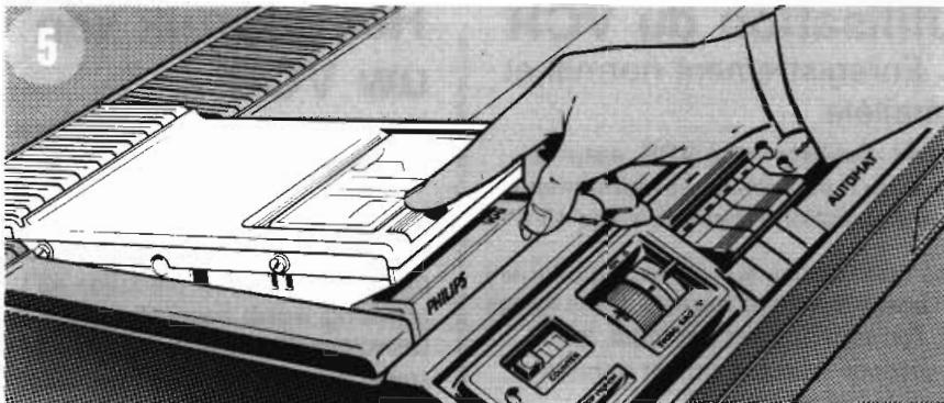
Press down on the ribbed plate of the cassette holder until the holder locks in position within the VCR.
