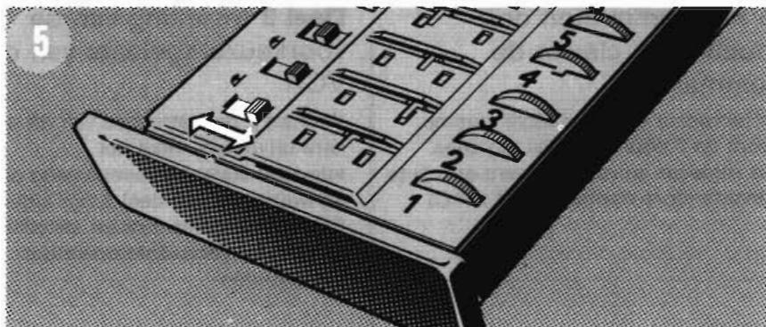
Set the slider switch of Tuning Control 1 on the VCR to the same group of channels as that of the first pre-selector control on the TV set.
