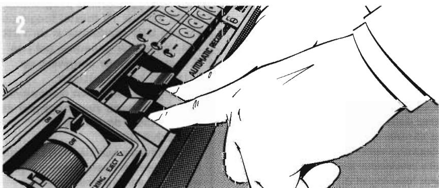
Simultaneously press the RECORD key and the START key.
