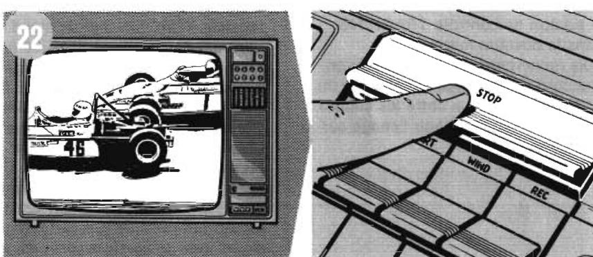
On the TV set, re-adjust the tuning control until another programme is shown on the TV set. Again check if the programme being shown is that of the test recording by pressing the STOP bar.
