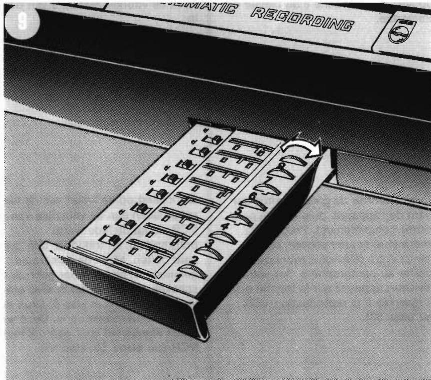
Adjust Tuning Wheel 8 on the VCR until the picture from the camera appears on the screen of the TV set. For further details refer to the instruction book of the video camera.
