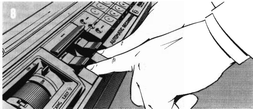
Press the RECORD key and the START key, simultaneously.
